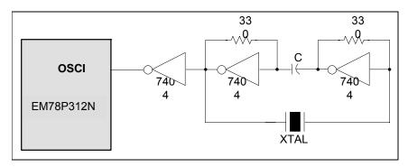
Fig. 5-31 Crystal/Resonator-Series Mode Circuit
